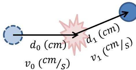
$$TOF (s) = \frac{d_0}{v_0} + \frac{d_1}{v_1}$$
