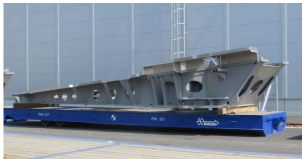
Fig. 2.8.1 REpower 5MW Fabricated main frame ready for assembly.
