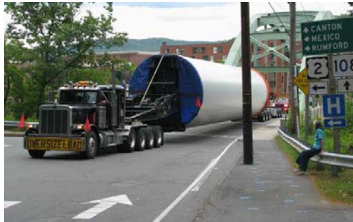
Fig. 2.2.6 Tower Transport by Truck
