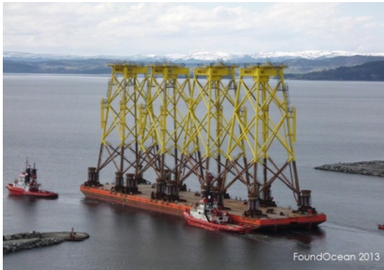
Fig. 2.5.7 – Traditional vertical transport of RWE jackets.
