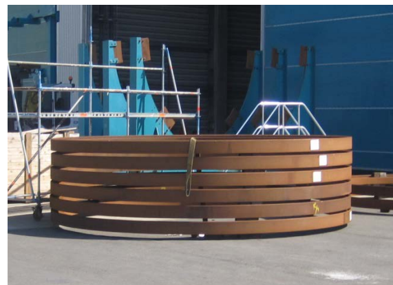
Fig. 2.11.2 Forged tower flanges ready for cleaning and tower assembly in Germany.
