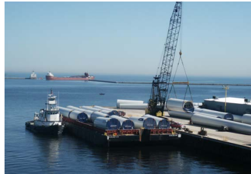
Fig. 2.2.7 Tower Transport by Barge
