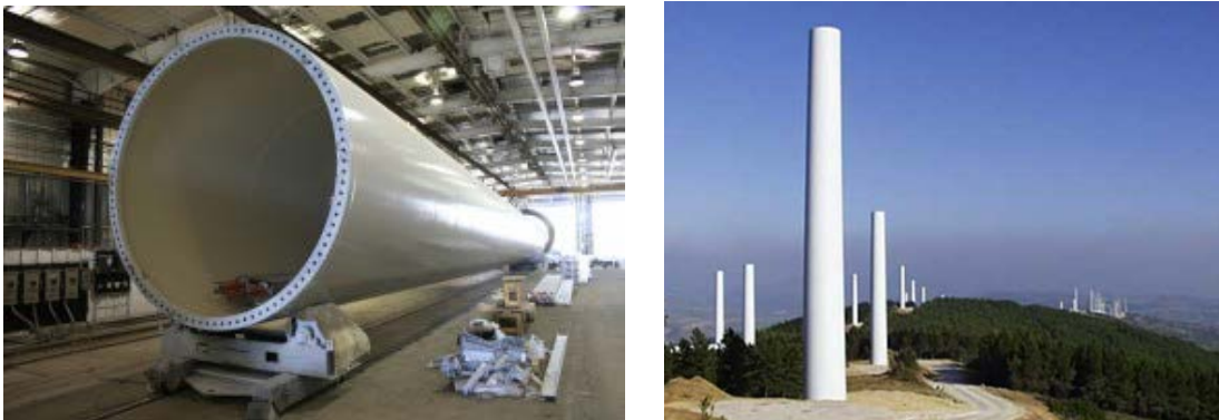
Fig. 1.1.1 Tower Section after Paint and Installed Towers
