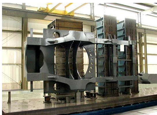
Fig. 2.8.2 K&M Machine Fabricators main frame in production
