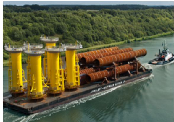
Fig. 2.6.7 Barge transport by Bilfinger Construction – London Array
