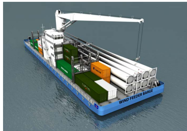
Fig. 2.3.7 Blade Transport by Barge
