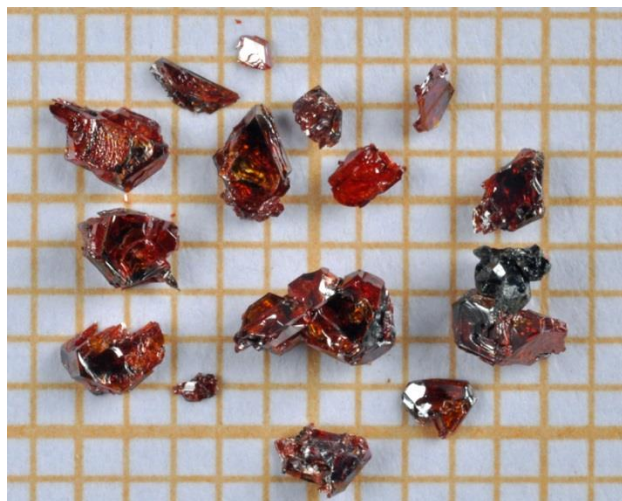
Figure 2 Optical macrograph of BP crystals precipitated from nickel-based. The grid scale is 1 mm.
