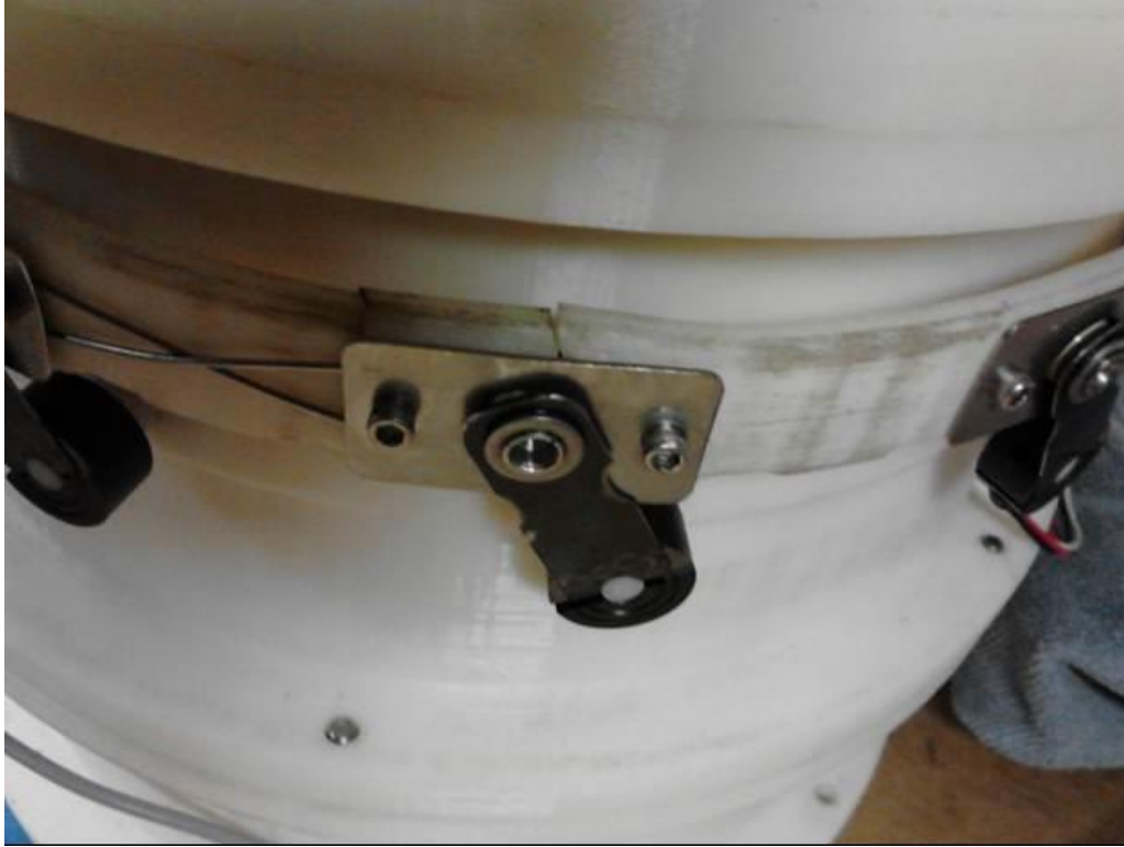
Figure 111. View of Damaged Shutter Valve Linkage
