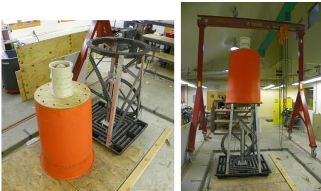
Figure 104. Dry-Turbine Test Apparatus Under Construction in CN 's Test Lab (Wilder, VT)
