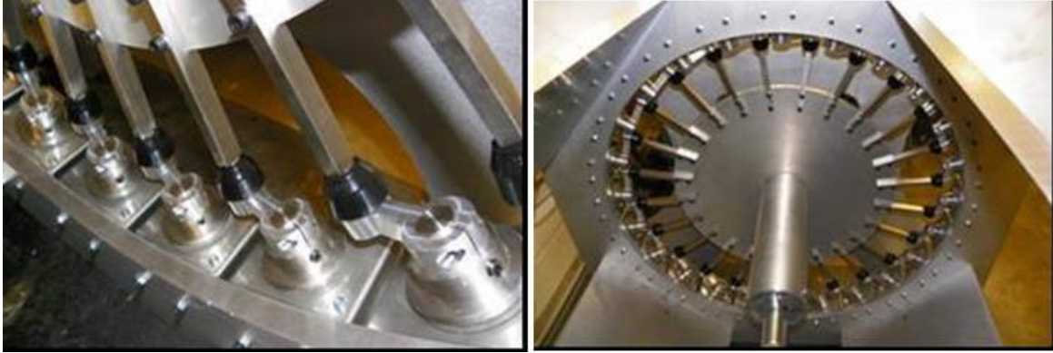
Figure 32. Construction of a Blade Stator Including a Blade Articulation System
