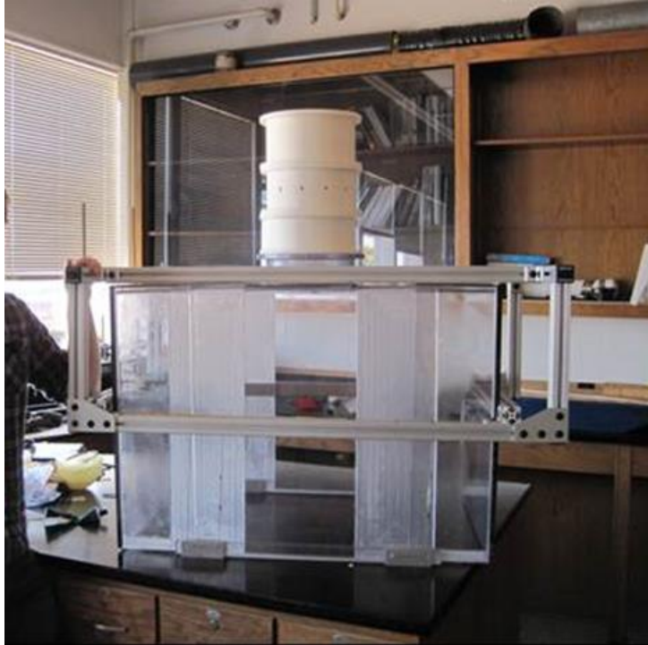
Figure 107. MMA Student Pictured with the Prototype OWC Structure Used with the Mini-OWC Turbine Water Wave Tests at the University of Maine
