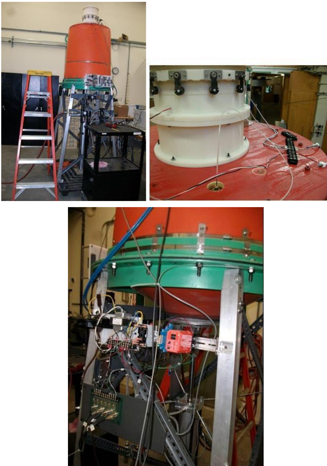
Figure 105. Dry-OWC Turbine Test Apparatus with Diaphragm Timing Circuit and Turbine (installed on top) in CN 's Test Facility (Wilder, VT)
