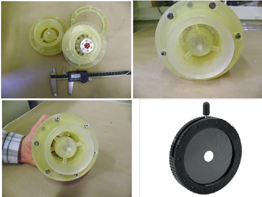
Figure 82. 10-watt Micro-OWC Turbine Prototype Assembly and Micro-Shutter Valve Used in the MMA In-Water Test
