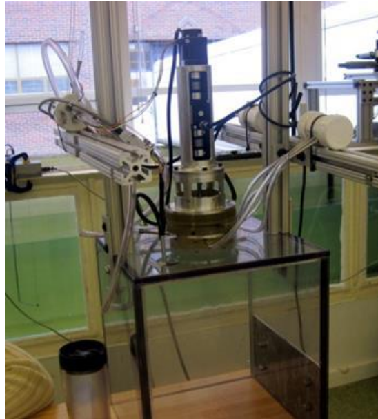
Figure 85. Micro-OWC Chamber with Torque Measuring System at MMA
