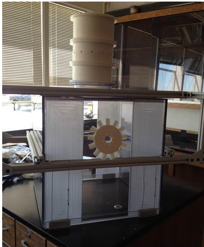
Figure 108. Prototype OWC with Adjustable End Sections Shown in Perspective with 200-mm Diameter Wells Turbine Rotor
