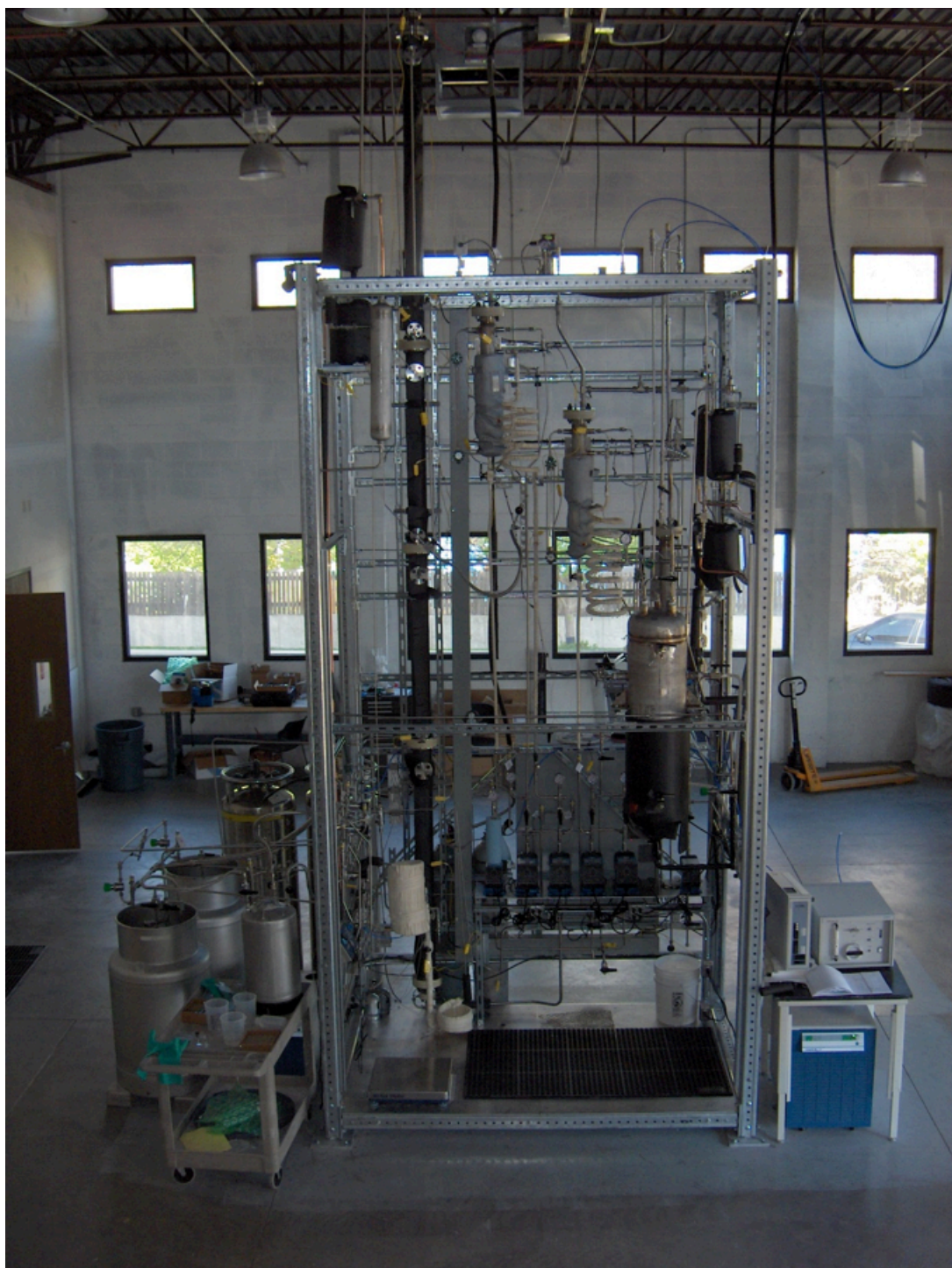
Figure 2: Image of ION's ~0.57 LPM continuous process lab test unit.
