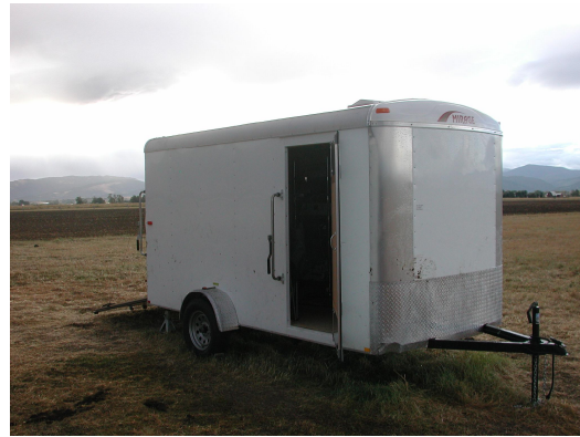
Figure 24 The cargo trailer housing the CO 2 DIAL instrument shown at its field
