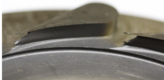
Figure 16: Turbine Nozzle with undercut; EDS sample location identified.
