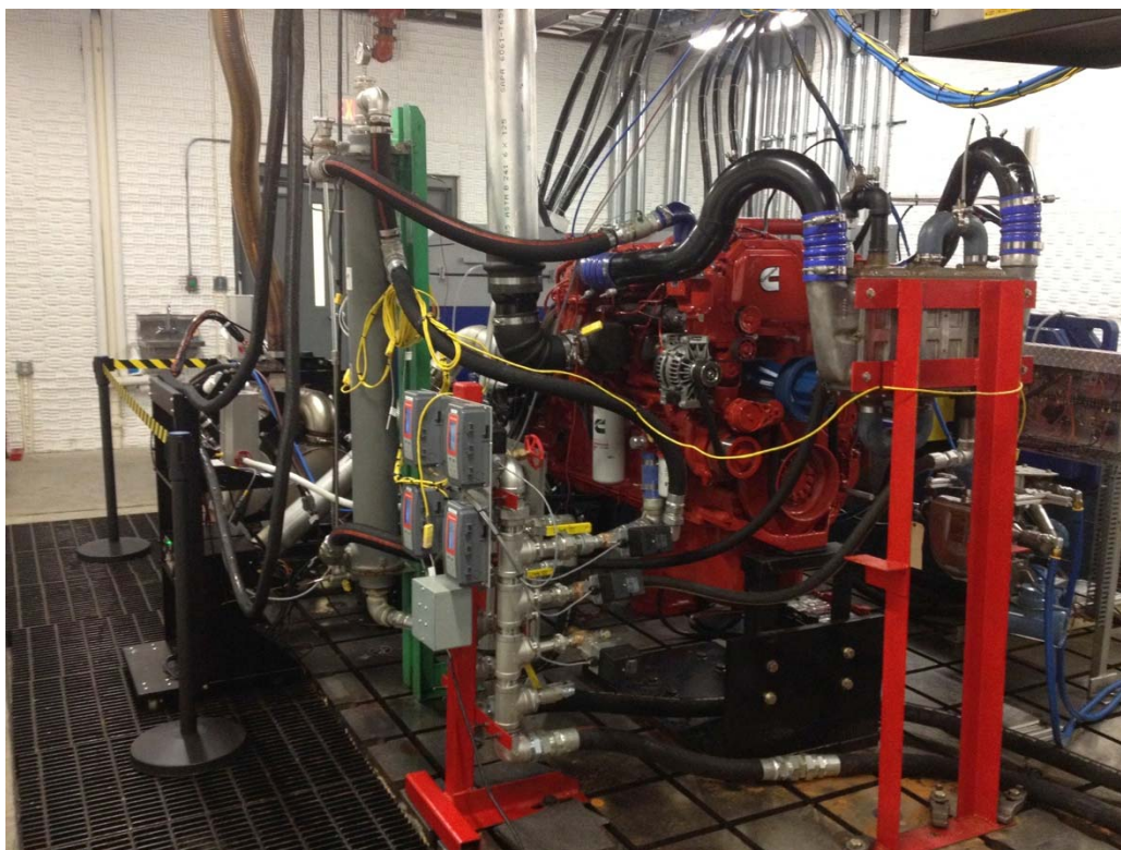
Figure 43 Engine-in-the-loop installation in the ORNL VSI Laboratory
