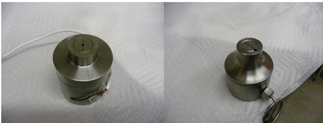
Figure 7-5 Images of the end caps (left: downstream cap, right: upstream cap)
