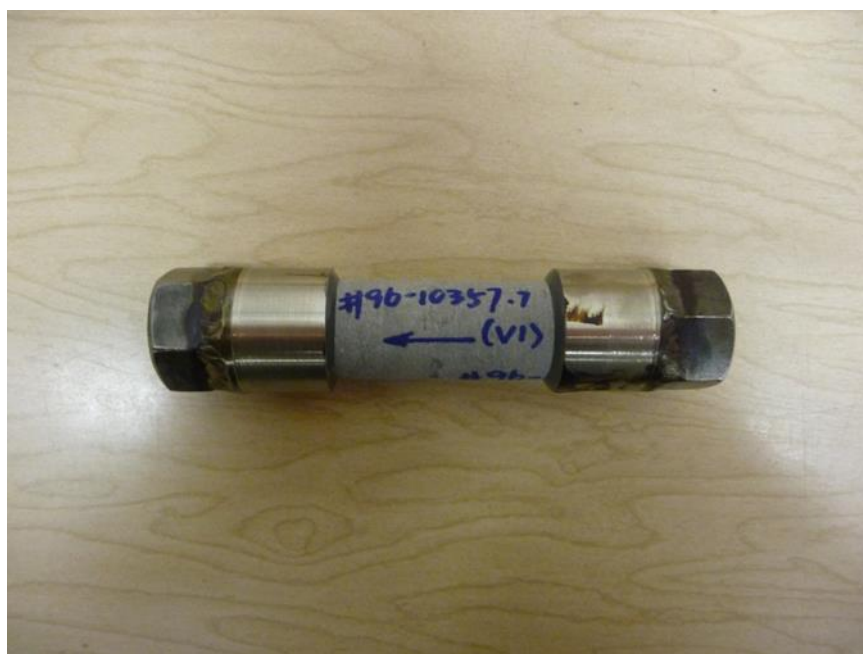
Figure 8-1. The preparation of core plug for tensile strength test
