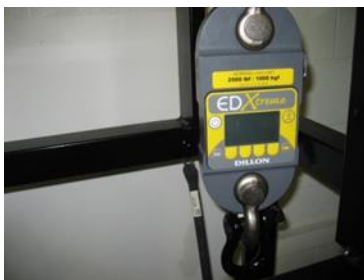
Figure 7-23. Dynamometer on top of tensile strength test apparatus
