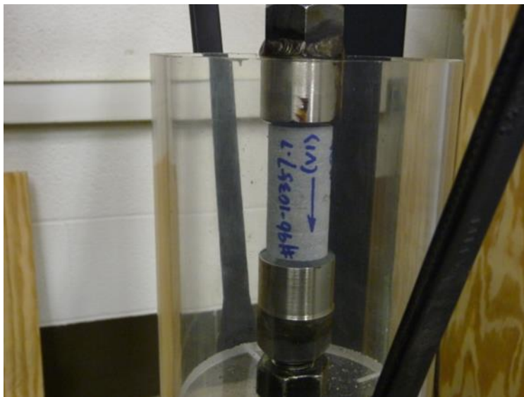
Figure 8-2 The installation of core plug on tensile strength test apparatus.
