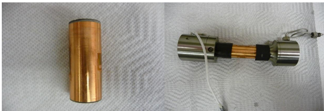
Figure 7-4 Images of core and core holder for rock properties test
