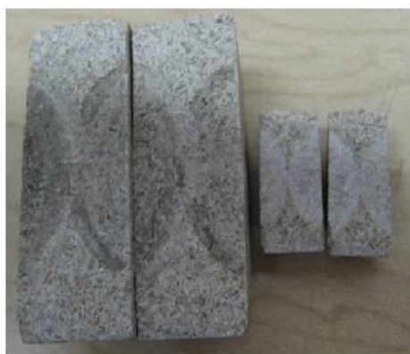
Figure 10-25. Both large and small samples (left) are in the valid geometrical range (right).
