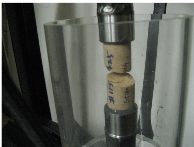
Figure 7-27. Specimen is crashed
