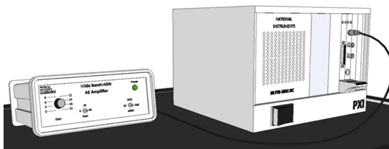
Figure 10-10. Wide band width amplifier (left) and NI Chassis (right) with a high-resolution digitizer and interface card installed.
