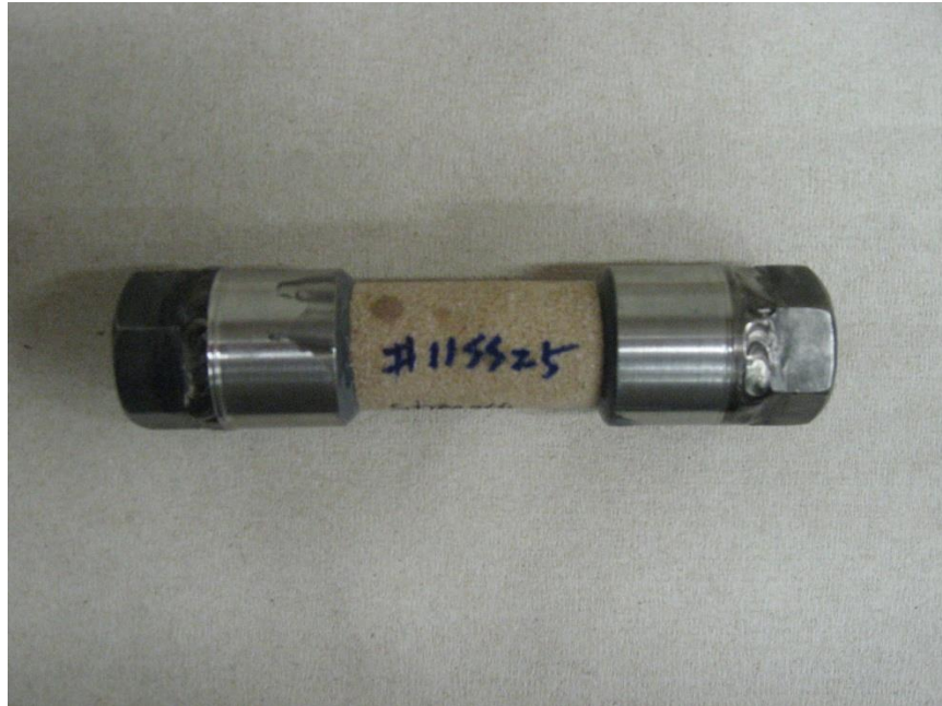
Figure 7-24. Specimen glued to steel caps
