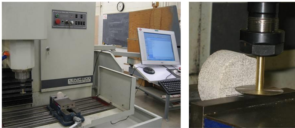
Figure 10-22. CCNBD specimen preparation
