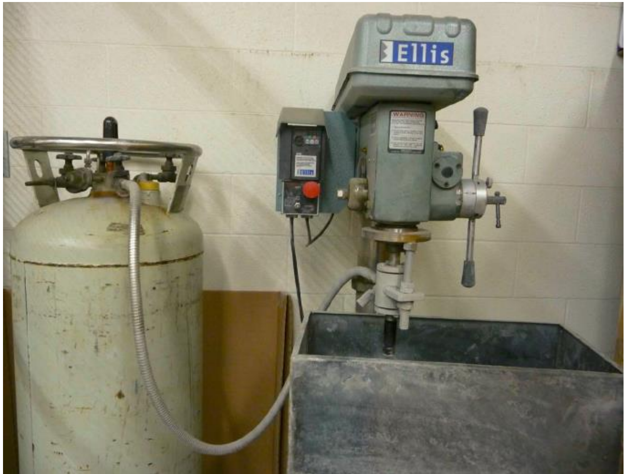
Figure 7- 1 Core plug sampling system used in this study
