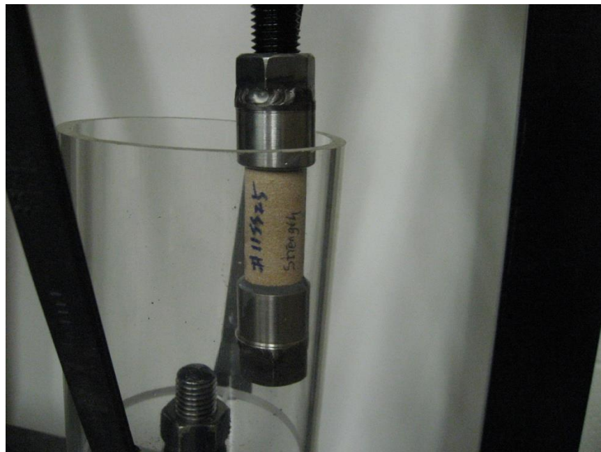
Figure 7-25. Tensile test apparatus (with upper side of the specimen is fixed)
