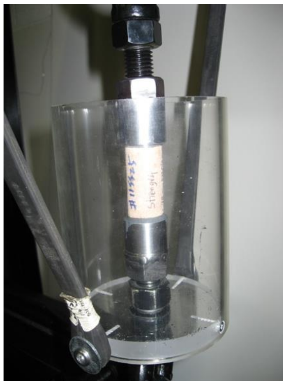
Figure 7-26. Tensile test apparatus (with both sides of the specimen was fixed)
