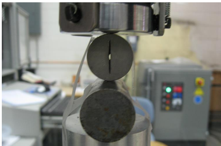
Figure 10-29. Shale sample under compression at MTS station
