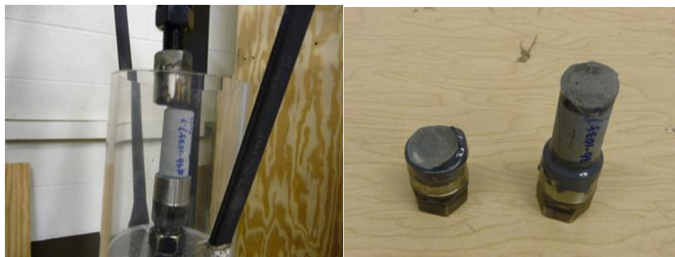
Figure 8-3 Pictures of the destruction of core plug after tensile strength test.
