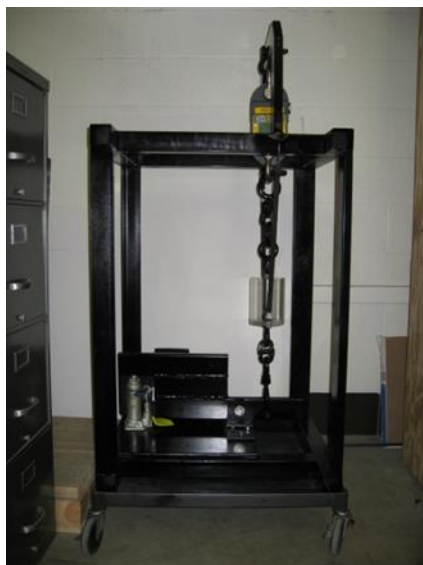
Figure 7-22. Tensile strength test apparatus
