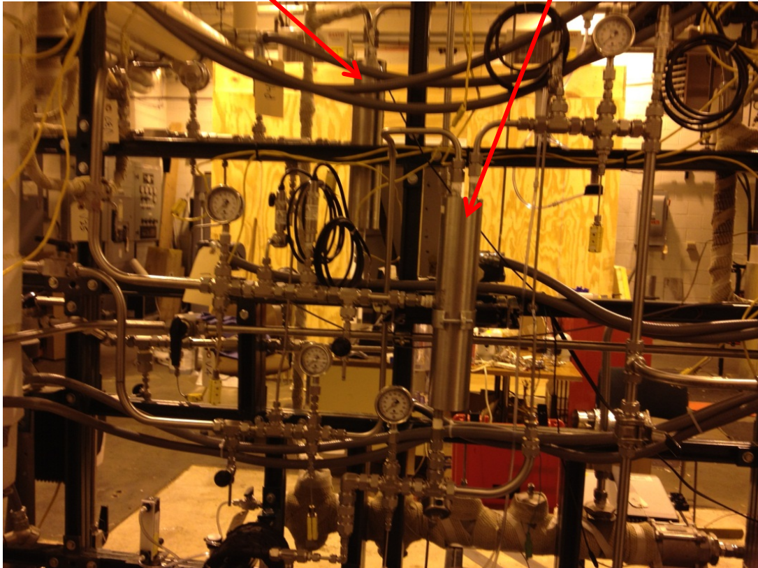
Figure 15. Photo of the membrane desorber unit. The membrane absorber unit is in the back section of the skid.
