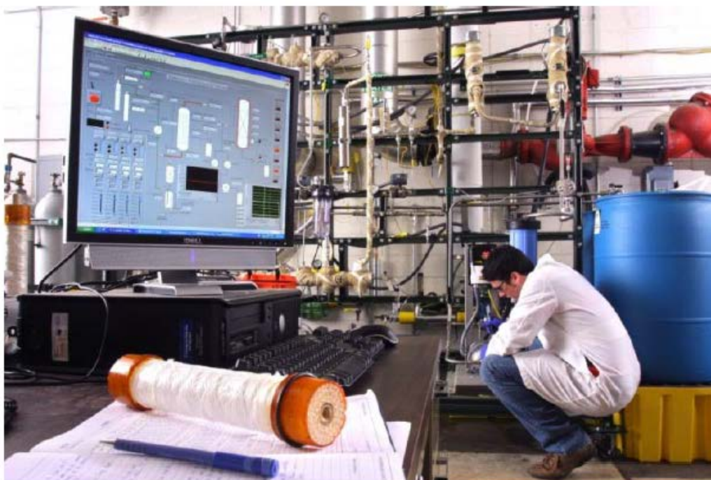
Figure 10. Photograph of the new post-combustion membrane contactor test apparatus.
