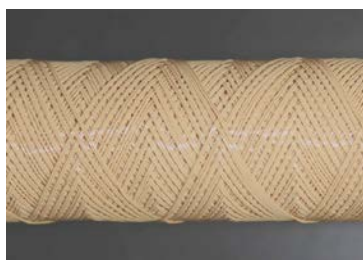
Figure 7. Helically wound structured hollow fiber cartridge.
