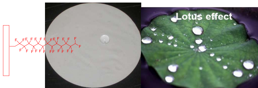
Figure 5. High contact angle and the non-wetting properties of porous PEEK membrane surface.
