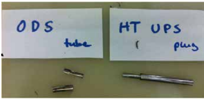
(e) ODS/HT-UPS welds and peel test
