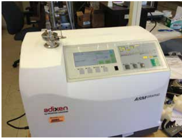
Figure 13. Set up for helium leak tests.
