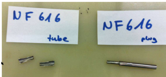
(c) NF616/NF616 welds and peel test
