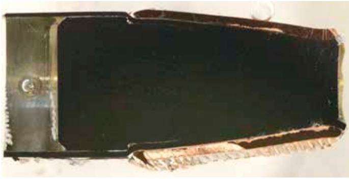
Figure 14. Cross-sectional samples in tube axis and radial directions, respectively.
