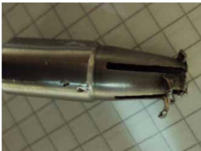
Figure 8. Tube/pin weld after mechanical peel test.
