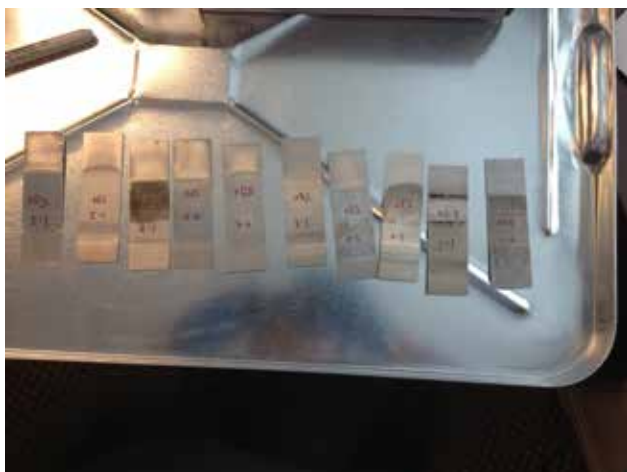
Figure 9. Examples of electro-polished and coated flat coupons.
