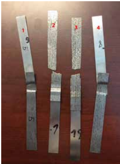
Figure 11. Tensile specimen of lap welds after tensile tests.
