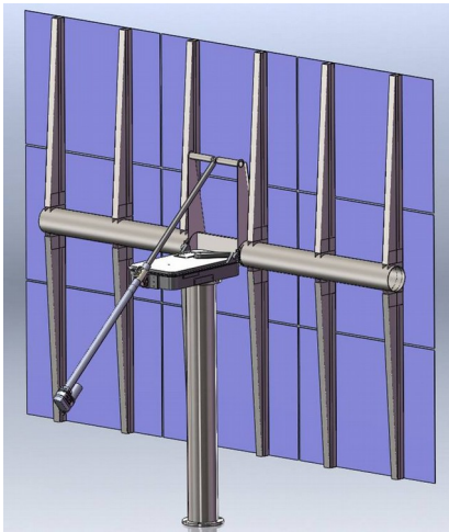
Figure 5 - 1st Concept with 36" Jack (left) and Final Concept with 18" Side Mounted Jack (right)
