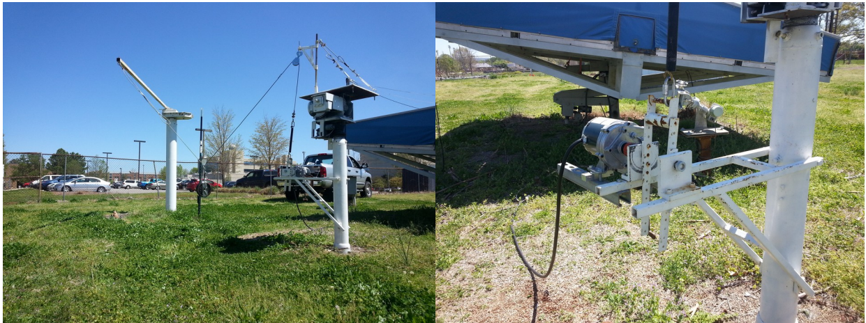
Figure 16 – Rig to Simulate Dynamic Loads (l) with close-up of vortex impulse load generator (r)
