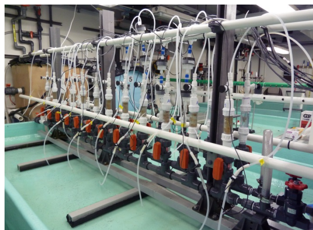
Fig. 7.2. Seawater manifold and PNNL style columns containing uranium adsorbent material.
