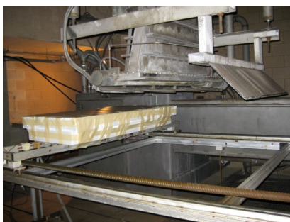
Fig. 4.4. Electron beam setup used for irradiating fiber samples.
