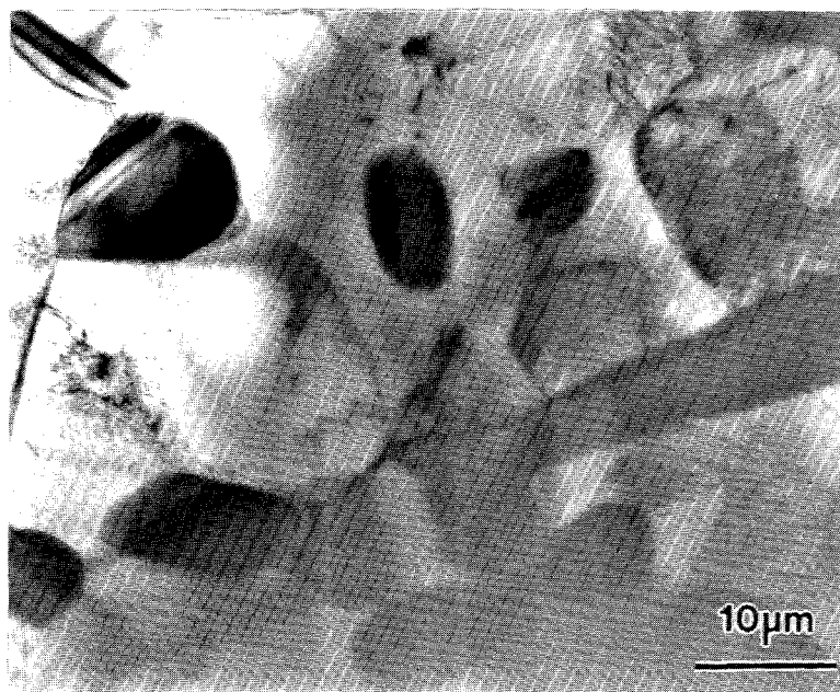
Fig. 4. TEM micrograph of CN-85 (Cr-Nb-1.5Al-5X1-4X2) hot extruded at 1480°C.
