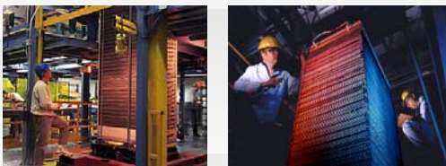
Internal fuel cell stack (similar in most systems) Individual fuel cells comprise a fuel cell stack
