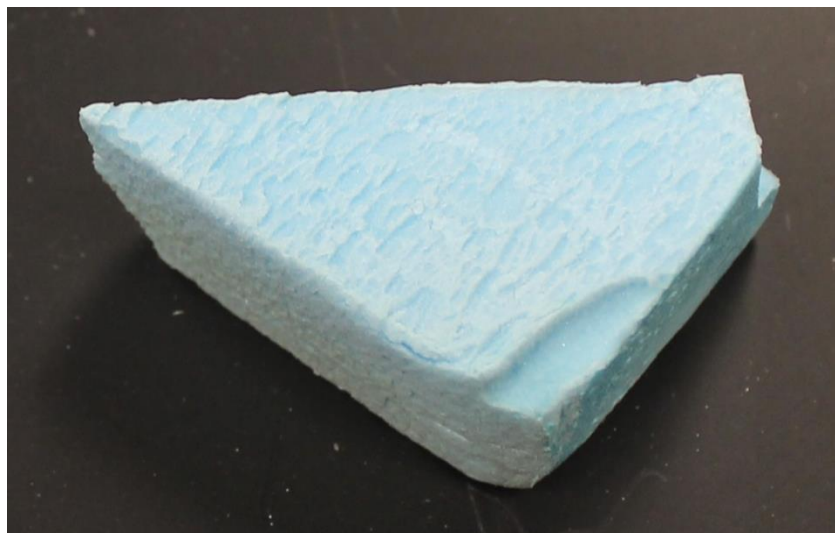
Figure 2. Picture of a small piece of the Dow Styrofoam™ Highload polystyrene foam before TGA analysis.
