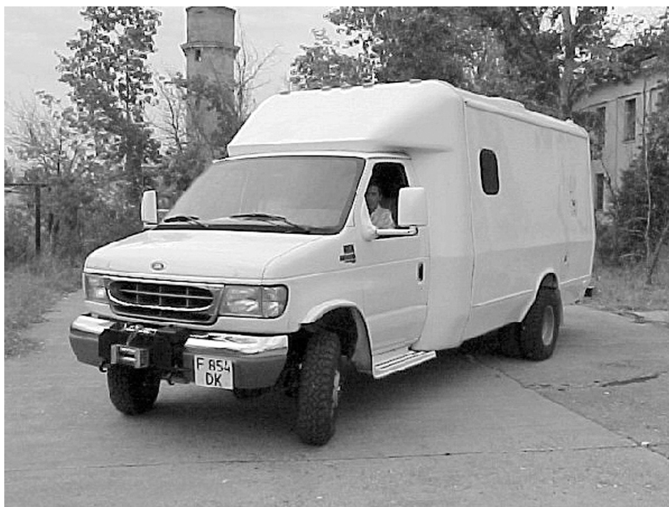
Figure 55. Mobile radiological laboratories complete with modern field \gamma -spectrometers, dosimetry equipment, and satellite navigation aids.
