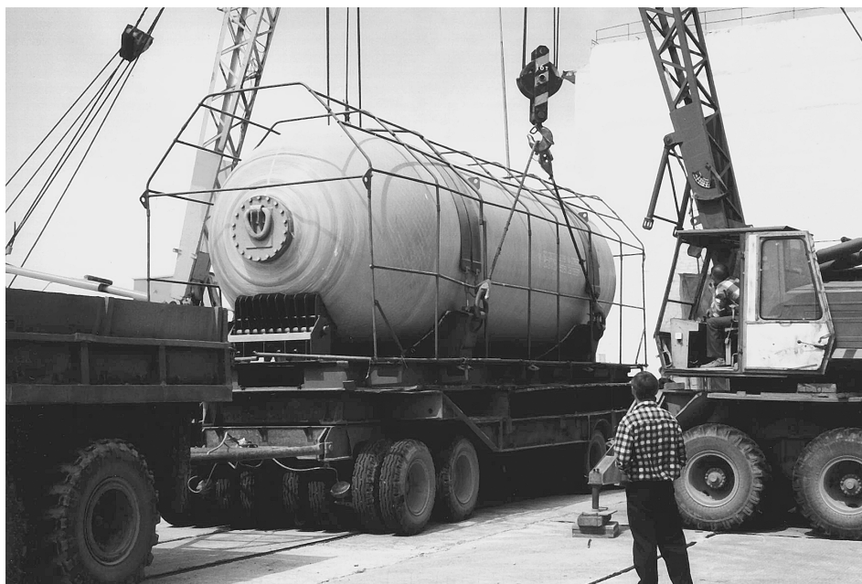
Figure 50. Exterior view of a flask container, mounted on a special carriage.
