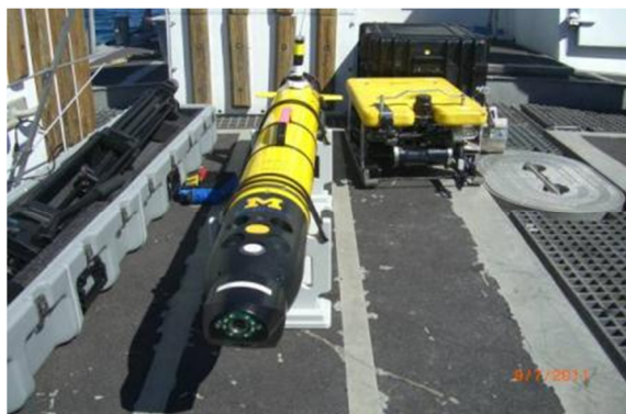
Figure 4 – UM's Iver 2 AUV and Outland 1000 ROV
