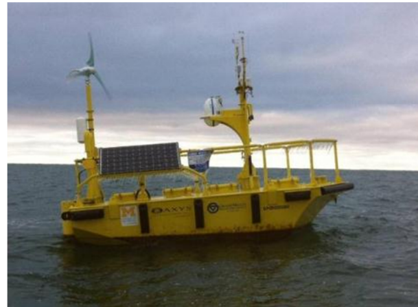
Figure 1 – WindSentinel Floating MET Facility
