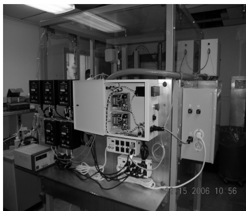
Fig.5 Process control and monitoring equipment mounted on the side of the acid decomposition skid.
