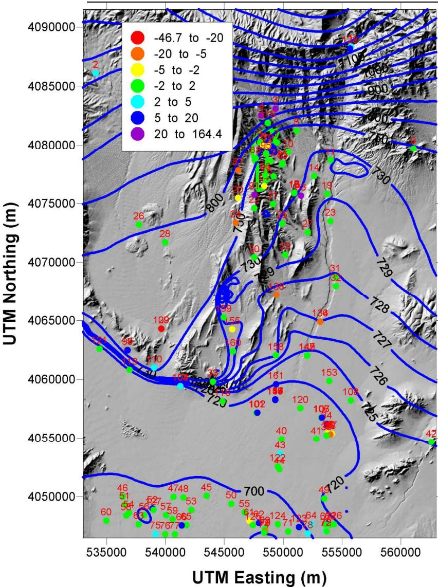
Heads along the model boundaries are extracted from the best estimate of the potentiometric surface, which is an update of previous potentiometric surfaces that now uses water-level altitudes measured through 2005
