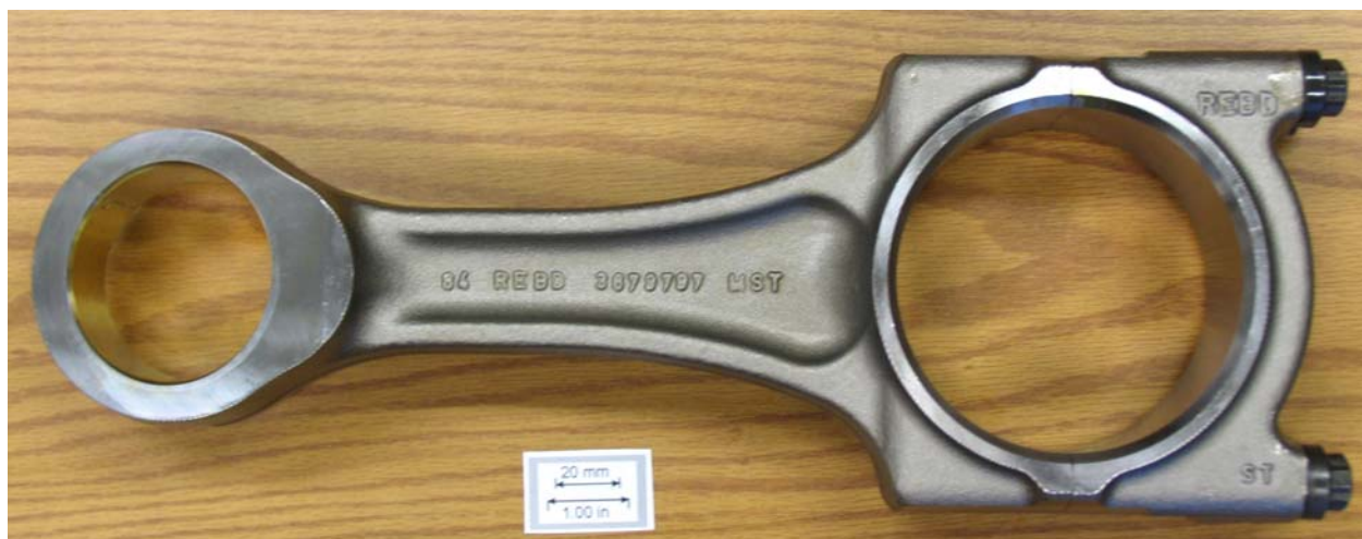
Figure 2. Commercial diesel engine connecting rod.
