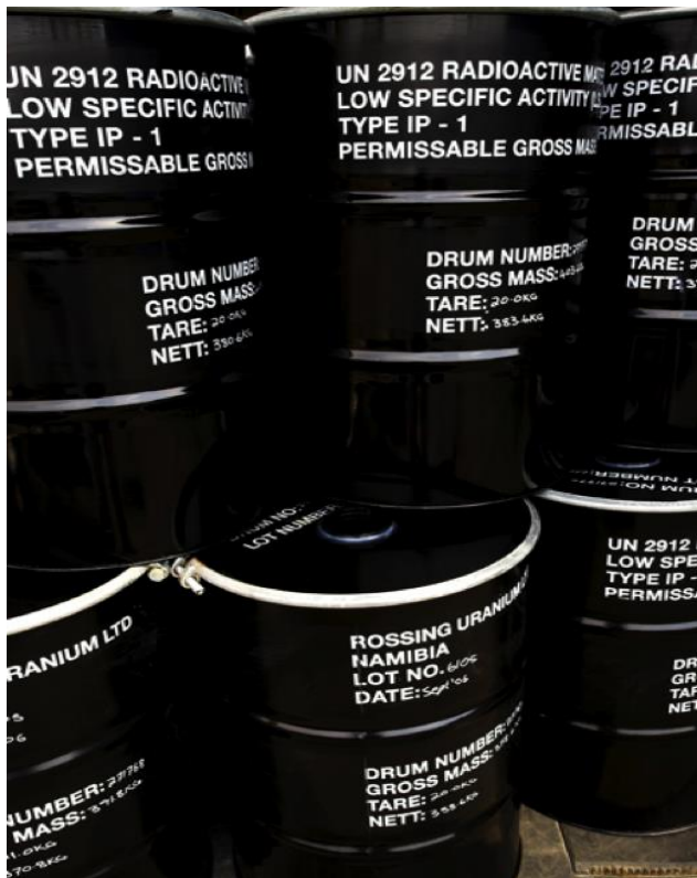
Figure 2: Drums of UOC with production details
