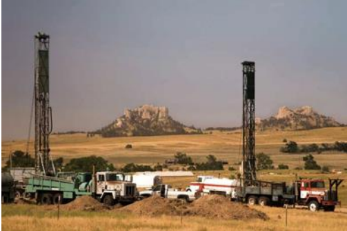
Figure 5: Drill rigs for core sampling
