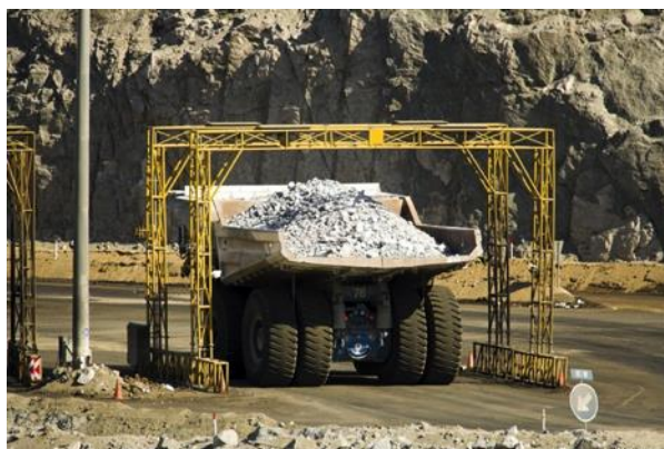
Figure 6: Gamma-ray detectors for sorting ore
