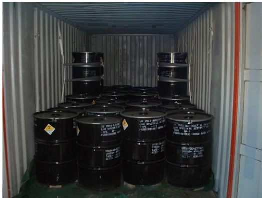
Figure 8: UOC drums loaded into a 20-foot ISO shipping container
