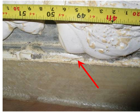
Figure 15: Crack in shear web to LP skin bond joint at 1.20-1.30 m on the CX-100 blade.
