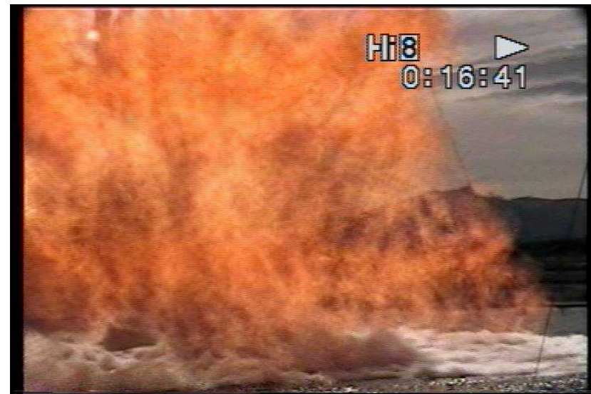
10 m LNG pool fire test on water performed at SNL, 2.5 m/s wind
