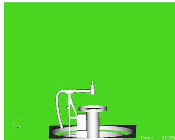
CFD simulation using FUEGO of 3 m JP-8 pool fire in Thermal Test Complex
