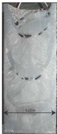
Figure 13: Image of siliced and etched ingot from current control test.
