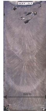
Figure 12: Image of sliced and etched ingot from Pool Power control test.
