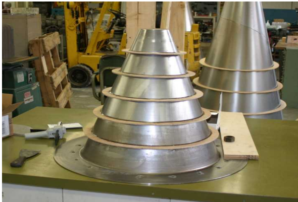
Stiffening rings mounted to PoP- RTL cone
