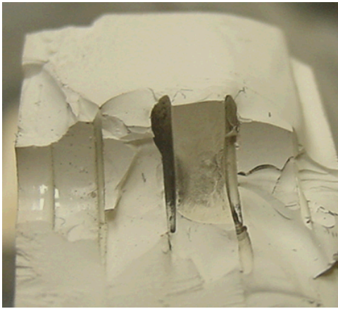
Figure 3. Dielectric material (electrodes removed) after device failure. Carbon on material adjacent to center electrode is evidence of partial discharge and/or arcing. In this device, the distance between electrodes was approximately 1.27mm.
