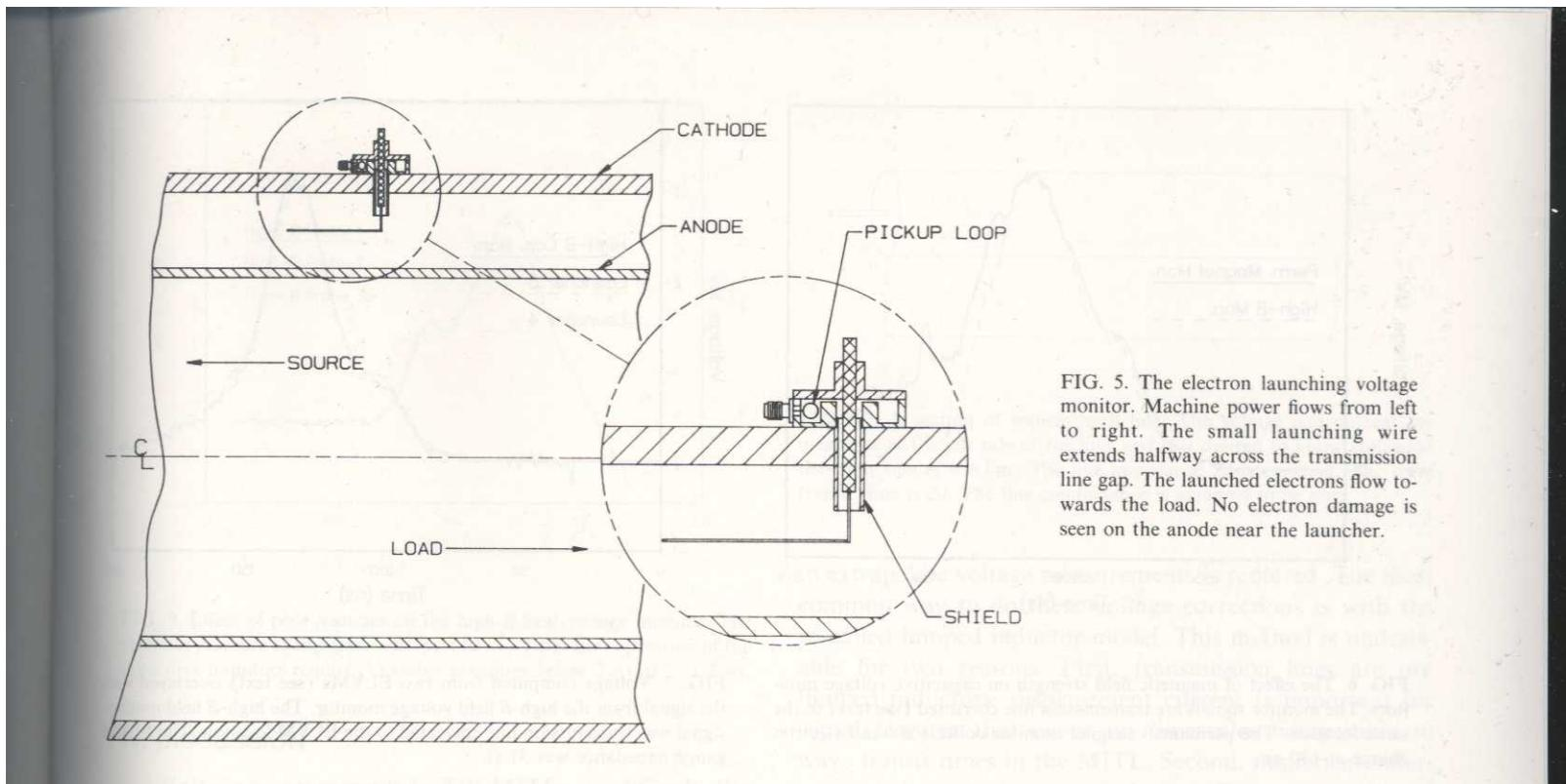
FIG. 5. The electron launching voltage monitor. Machine power flows from left to right. The small launching wire extends halfway across the transmission line gap. The launched electrons flow towards the load. No electron damage is seen on the anode near the launcher.
