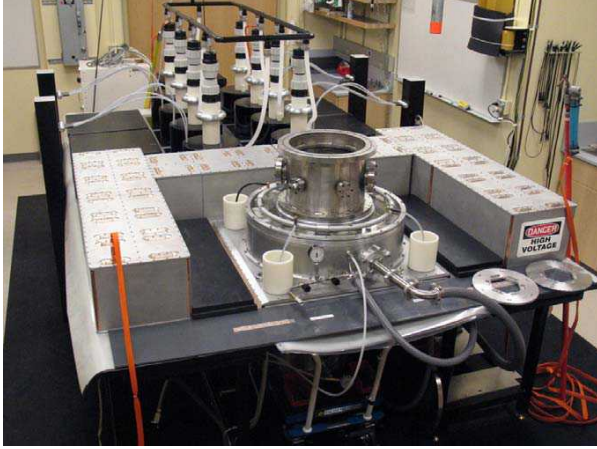
Figure 2. The WSU pulser located at the Institute for Shock Physics. The main capacitors are in the background, and the peaking capacitors surround the cylindrical load region in the foreground.
