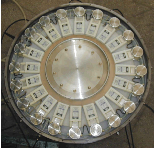
Figure 2: 500-kA LTD cavity designed at the High Current Electronics Institute. Current from 20 ‘bricks’ are added in parallel to provide a 500-kA current pulse.
