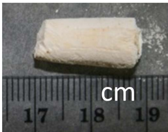
Figure 11. An optical photograph of an ice-templated \text{CeO}_2 structure prior to sintering.
