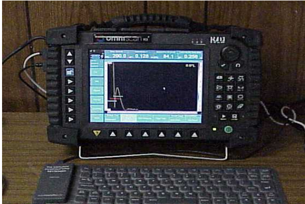
OMNI Scan UT Inspection Unit ( 10 MHz Phased Array Probe)
