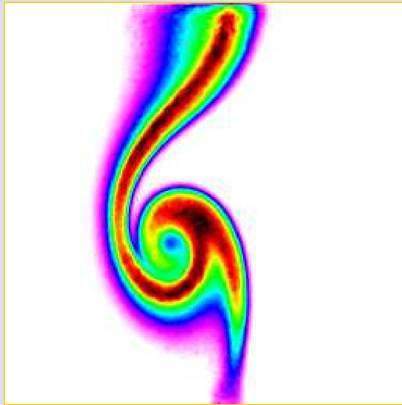
Planar LIF image of CO in flame (CRF Advanced Imaging Laboratory)
