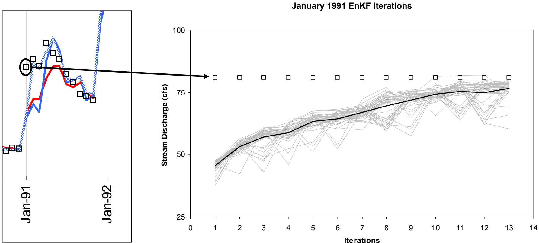
13 iterations to achieve a tolerance of 5 cfs
