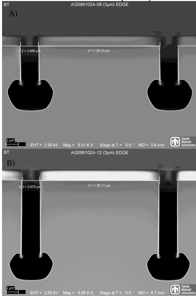
Figure 5: Cross-sections of channels formed using CDE etching after trench formation. The side walls were protected with 1000A of LPCVD oxide. A) Using a 3 \mu m wide trech that was originally 5 \mu m deep. B) Using 3 \mu m wide trech that was originally 10 \mu m deep.
