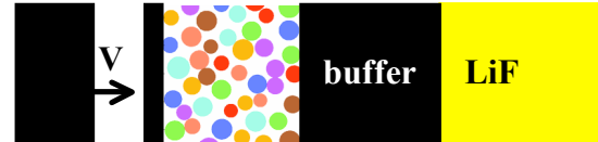
Figure 3 Setup for the mesoscale model. Periodic boundary conditions used on top and bottom.
