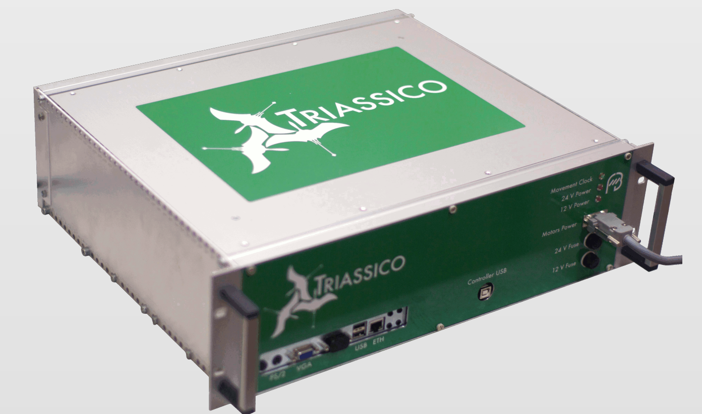
Figure : Controller rack of the system. It has an embedded computer for the movements calculations.
