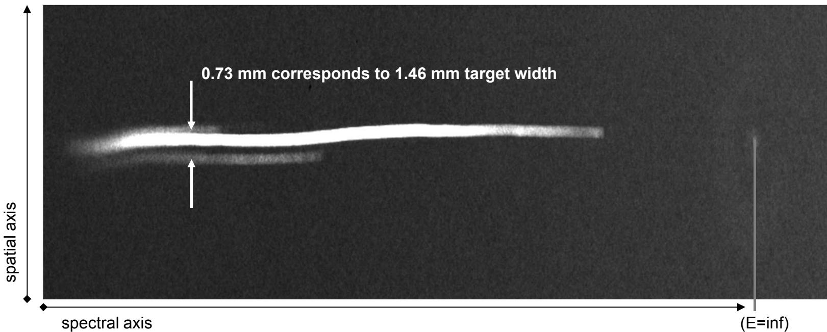
Low energy protons are emitted from the edges of the target foil and leave parallel ghost images on the image plate behind the Thomson parabola. Similar to X-ray emission, the intensity is substantial due to field enhancement at an edge. The entrance pinhole of the spectrometer projects a 1:2 demagnified 1D-image of the source.
