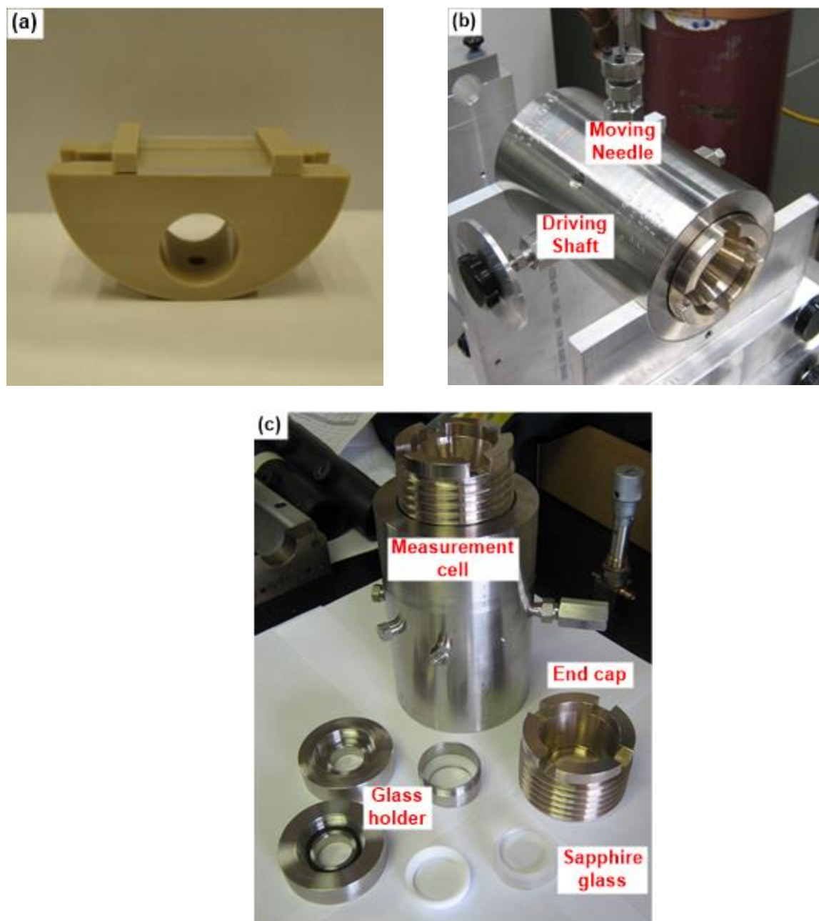
Figure 3: IFT/CA measurement cell: (a) crystal holder, (b) driving shafts, (c) the cell components.
