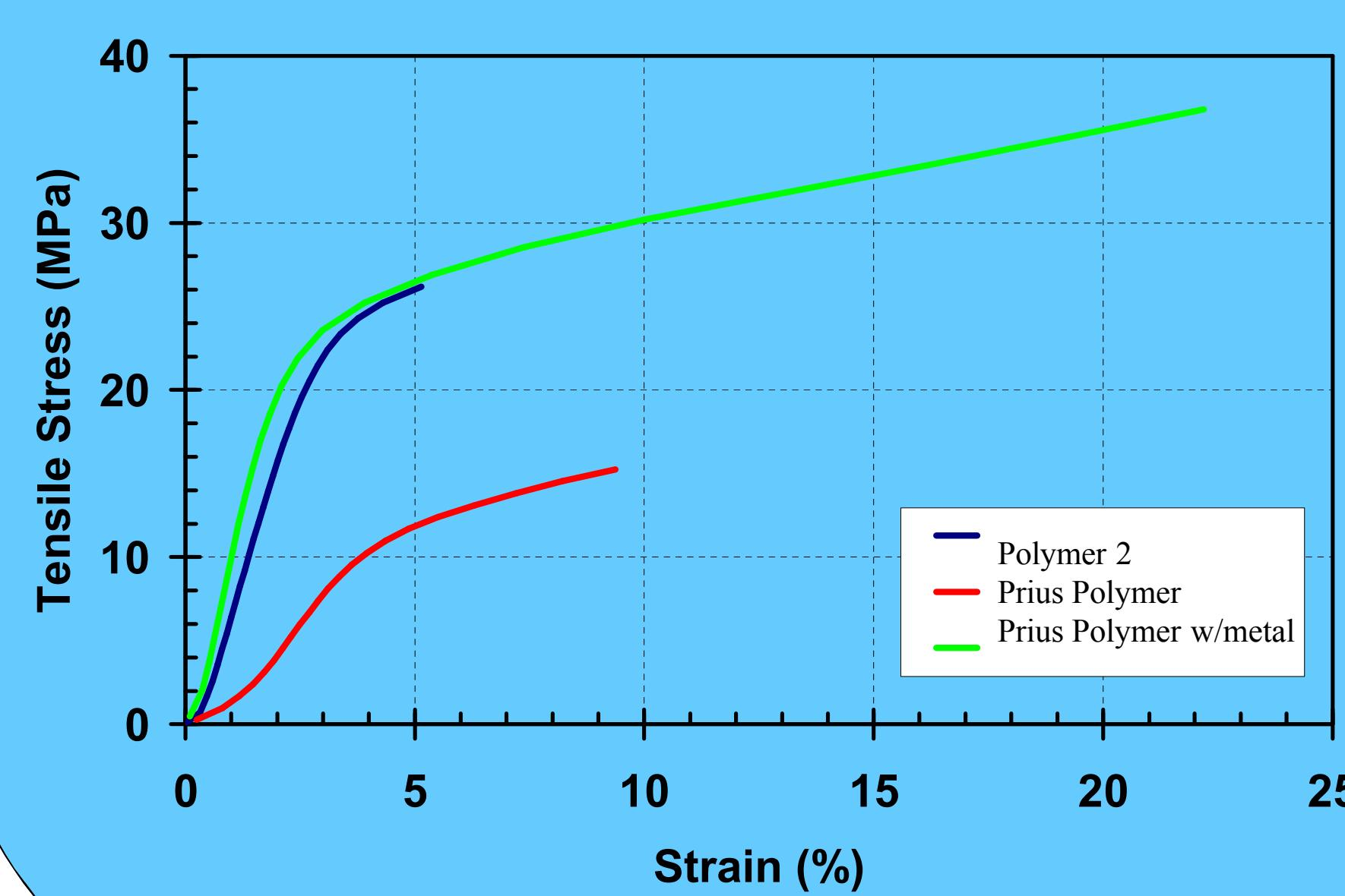
Tests were run in the TA DMA using the film grips with a loading rate of 3N/min. The samples were cut with edges that were not very parallel
