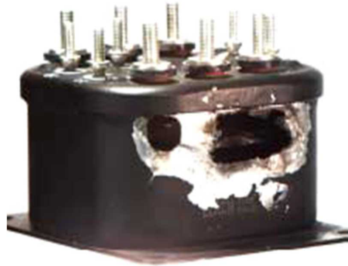
Whisker induced plasma arcing. Courtesy: Gordon Davy, Northrop Grumman
