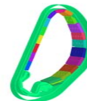
10° sector model of all 18 SM for electromagnetic analysis
