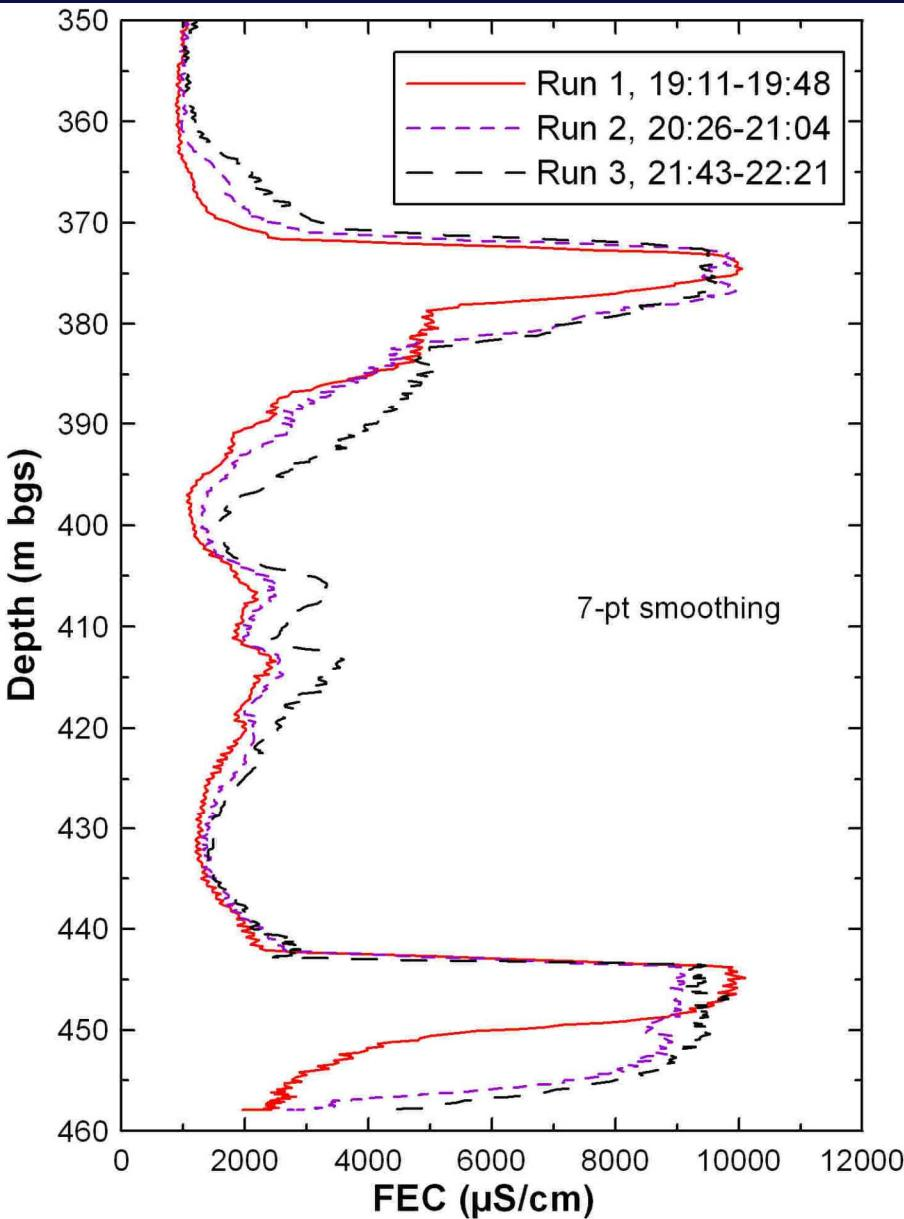
**The FEC spikes at ~373 m (A0 Member of Salina Formation) and ~443 m (lower Manitoulin Formation) moved only downward, reflecting sinking of dense fluid**
