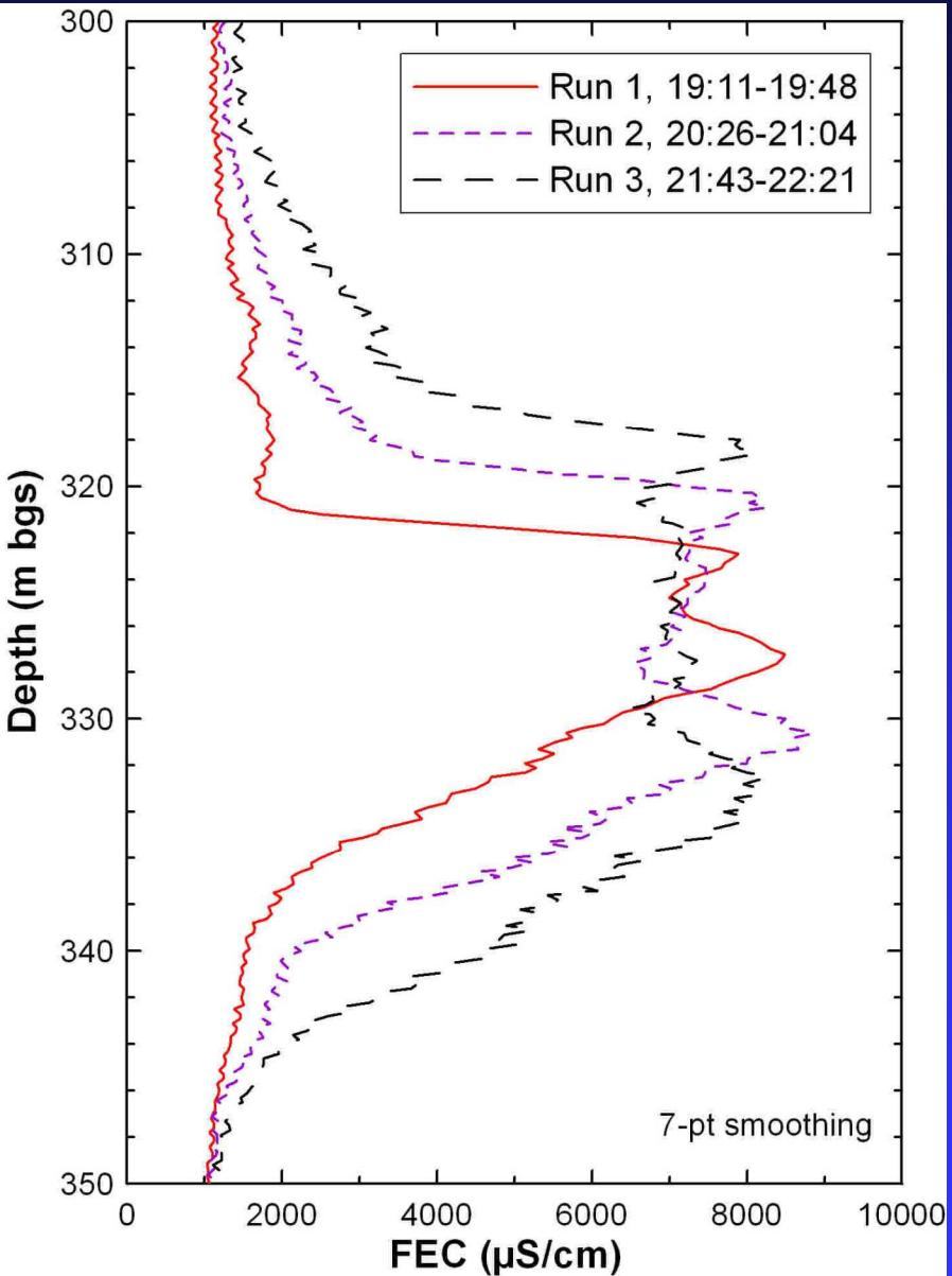
**The FEC spike at ~322 m (lower A2 Member of Salina Formation) spread both upward and downward with time, probably reflecting both upward flow and sinking of dense fluid**
