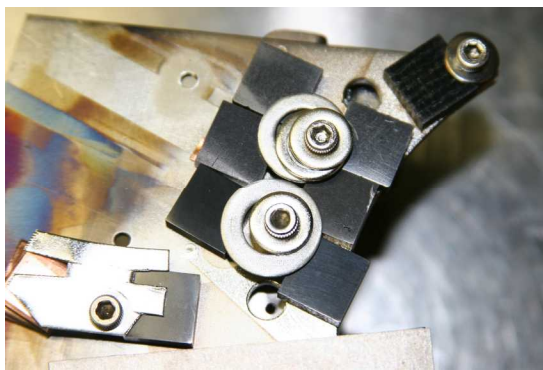
Samples mounted for higher fluence compared to C400 (Below). Tungsten shields extend towards beam center (right)
