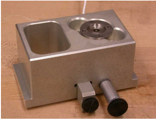
Picture of in-situ biaxial stressing fixture
