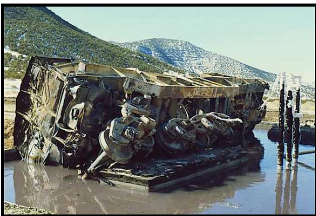
Fig. 8. Cask/Railcar following exposure to fire for 125 minutes.
