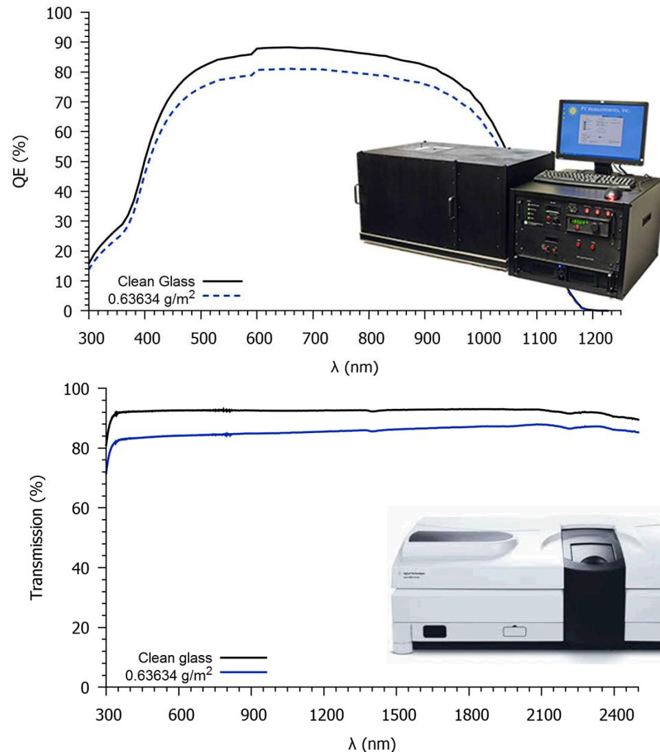
Goal is to apply indoor measurements and artificial soiling technique to determine a minimum detectable level of soil
