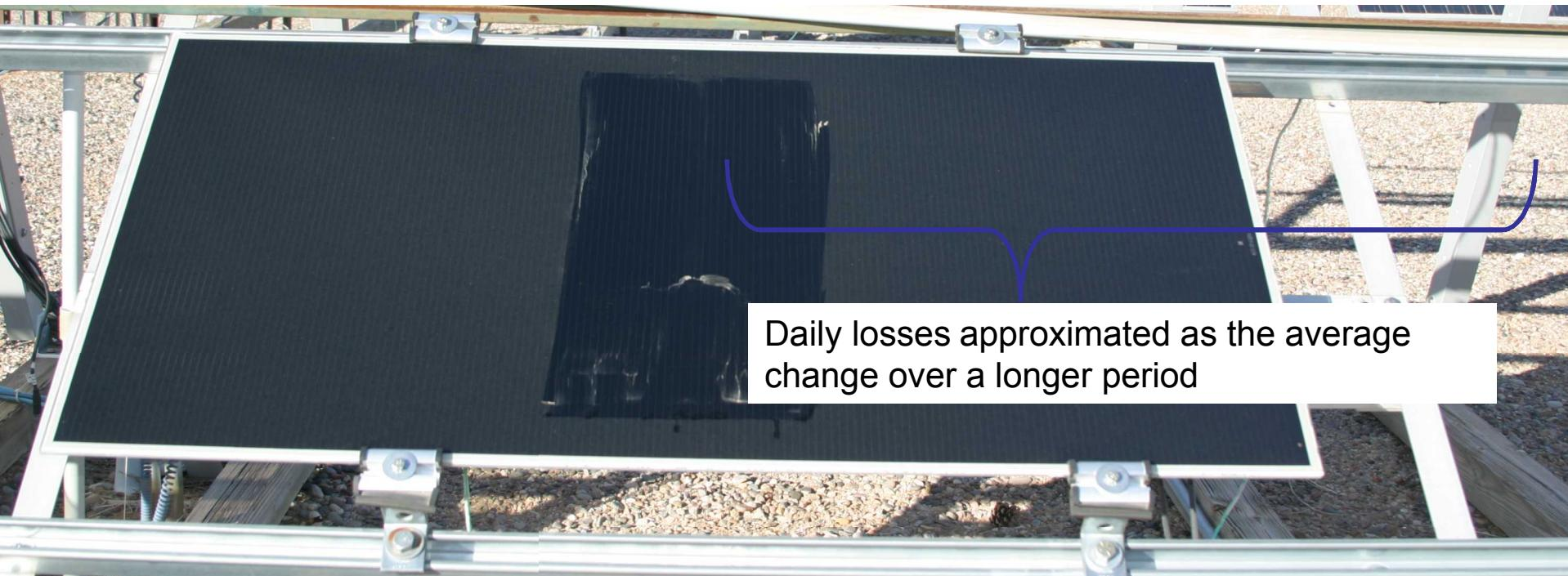
**A quantifiable limit is needed to better understand the effect of light soil accumulation on PV modules.**
