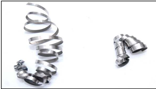
Free machining vs. Extrusion machining
