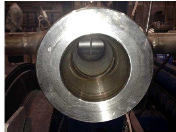
No evidence of overheating, fittings properly aligned, 3 weld passes, even penetration, no concavity
