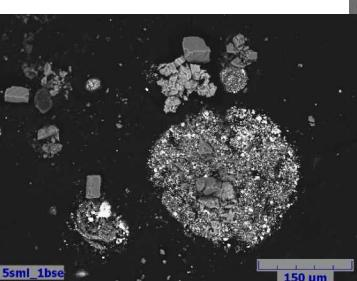
Shock sinter to become large particles
